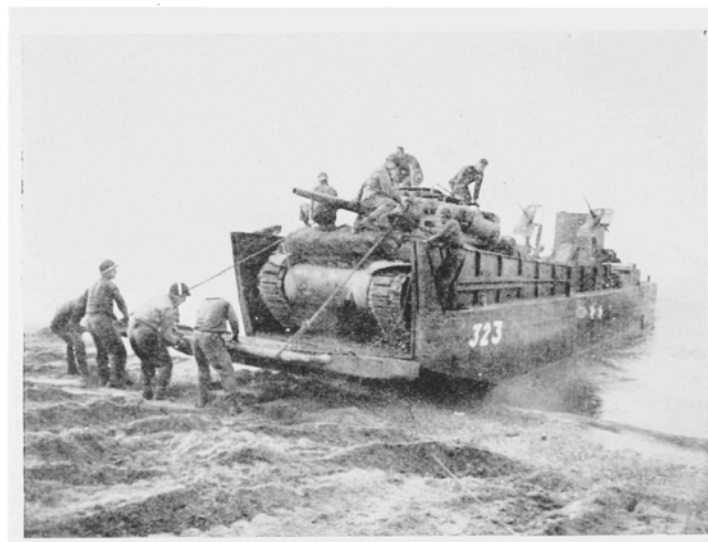
CLOSING DAMAGED END RAMP ON LCM BY MEANS OF ROPES ATTACHED TO M4 TANK
